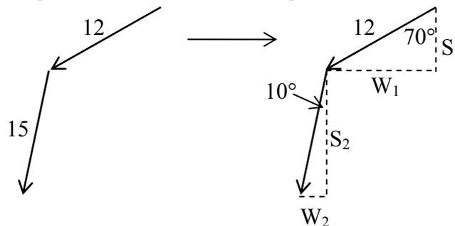
The distance West of the starting point is:  $W_1 + W_2 = \sin 70^\circ \times 12 + \sin 10^\circ \times 15$
